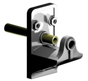
Locate a 6mm length of 1mm brass tube into the centre of the plate. Ensure that the front face is clean and square. The face lever and counter weight are located in the middle of the gap. The tube at the rear of the plate should be located in but not through the post, drill a 1 mm hole into the front of the post.
