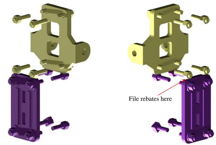
The 2<sup>nd</sup> lamp bracket (with lamp attached) can be test fitted to the 1<sup>st</sup> bracket and adjusted to suit. The ideal position for the position of the lens is in the middle of the spectacle plate , and the mounting of the bracket is critical for this to be correct. *See Assembly - 8*
