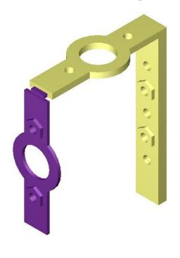
Once folded, solder the laminated bracket together and clean up. Clean out all small holes with an 0.4mm drill, and the large hole with a 1.5mm drill.
