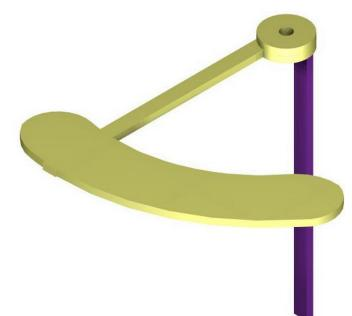
The extension is folded under and laminated. Clamp the part so that it is exactly under the original etch, and solder the parts together.
