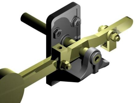
As an alternative to Scale Hardware nut and bolts. The hex and plain etched washers on the nickel silver fret, can also be used, in conjunction with 0.4 mm brass wire. You will need to be careful when gluing or soldering as you need the clevises to be able to pivot when assembled.
