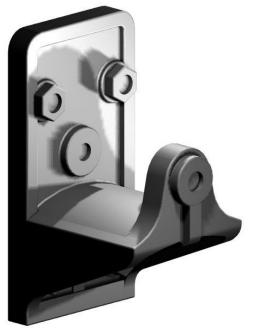
The lever face plate is bolted through the signal post and has the face lever and counter weight pivoting through the centre. The rod from the signal box is connected to the face lever, which in turn is connected to the signal arm.
