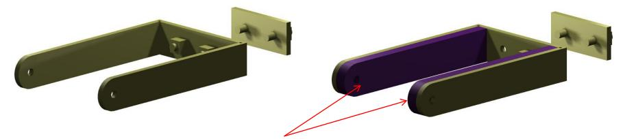
These holes need to be drilled out after being glued inside the landing etch.
