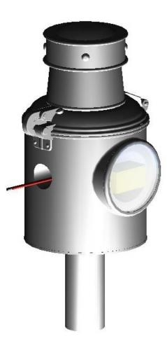
Fit an 0.8mm Golden White LED to the lamp. Feed the wires through the 1mm holes in the side of then lamp. Use a clear adhesive to hold the LED in place (supa glue or araldite), and to also keep the leads from shorting against the lamp.
