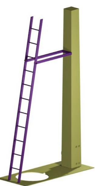
The ladder standoff is attached to the post using your preferred method,( shown here with square simulated nuts) the ladder is bolted to the stand off using 0.5mm threaded nuts and bolts, or etched washers and wire rod, and the ladder has the base soldered into the slots provided.
