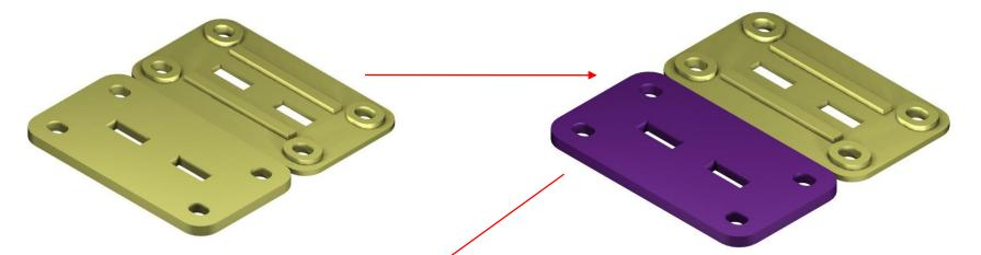
The signal bracket is a simple laminated etch folded 180 degrees and soldered together, cleaned up and washed in warm soapy water. Use peg clamps to hold the folds together while soldering.
