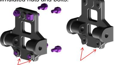
Small rebates can be filed into the base of the casting to allow the bolts from other parts to be fitted in place without interference.
