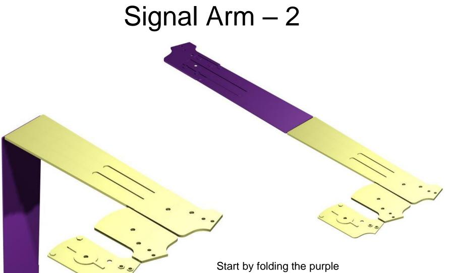
section down and the back underneath the main arm section
