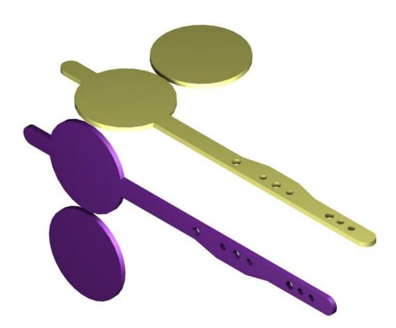
If the small tabs are broken there is a plan "B" which includes locating the parts with sections of brass wire through the holes in the arms and soldering the parts together with them aligned.
