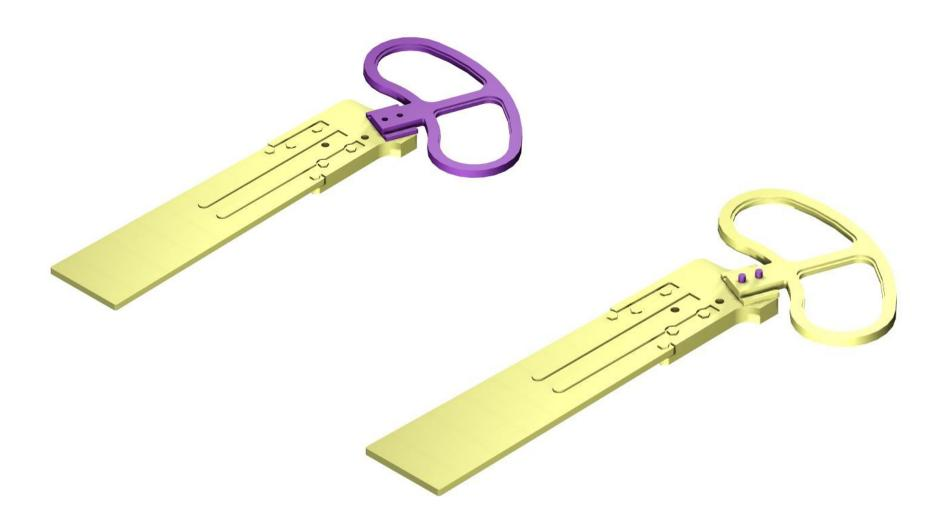
When soldering the spectacle plate to the arm, locate the plate with wires, and solder the parts together, being careful not to use excessive solder and fill detail.
