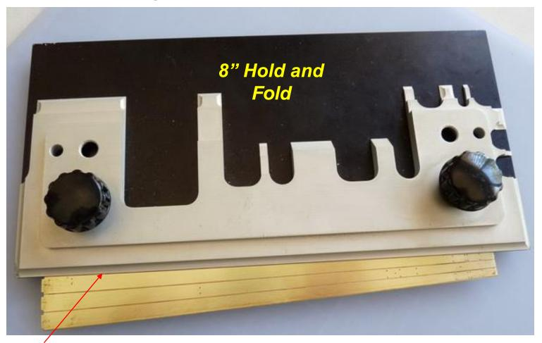
The fold line needs to be exposed approximately ½ to ¾ of the line. If the fold line is not exposed the etch will crack, and will be in need of repair. You can fold the etch just a tad past 90 degrees and allow it to spring back.
