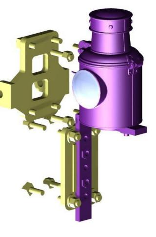
The first graphic shows the lamp with the lens slightly to the left of the spectacle plate, this position, is not correct and needs to be rectified • •
