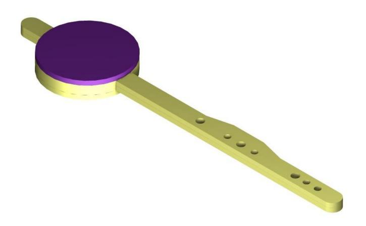
Once soldered together, the parts require cleaning up and the holes can be cleaned out using metric number drills.
