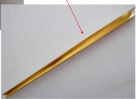
The use of cheap bulldog clips can assist the clamping and soldering of the post . Start from the base and work your way to the top, moving the clamps as you go, remember that the sides will fit neatly into the rebates of the etch.
