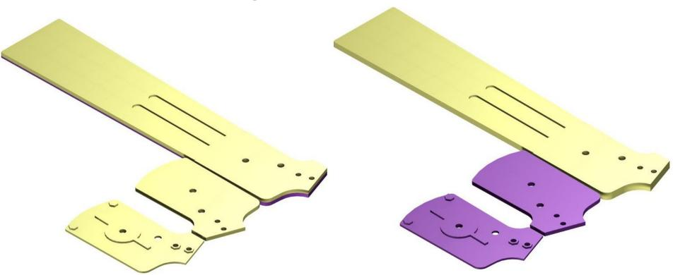
Next fold the small boss sections over onto the top of the main arm section.
