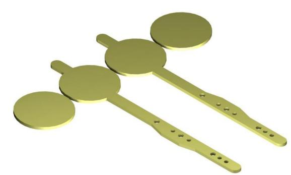
The Counter Balance Arm, needs to be folder 180 degrees, to form a solid laminated arm, There is a small ring on the outside of each segment which is NOT used and can be removed.
