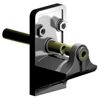
Locate a 2mm length (longer and remove the excess) of 1mm brass tube into the centre of the boss at the front of the plate, make sure that the face of the tube is clean and square. The gap left should be approx 0.6mm to locate the Face lever and counterweight. The wire pivot should be 0.5mm. The tighter the better (within reason). It is your choice. You can use the assembled counter balance to help locate the tubes.
