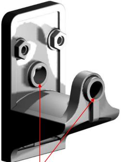
Drill the centre pivot 1 mm. Start by drilling a 0.5mm hole and open the hole up to 1mm. Ensure that the hole is drilled squarely to the plate.
