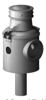
The signal lamp as supplied, it has a dimple in the centre of the lens to allow starting of a drill for drilling out the centre for an LED (not supplied) The spigot at the base of the lamp needs to be reduced to a diameter of 1.5mm.
