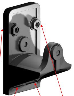
The bottom holes are drilled 0.4mm. Locate the plate on the signal post and drill the top holes through the signal post into the rear of the face plate. The holes should be accurately located, but by coming through the post the plate should end up sitting square on the post.
