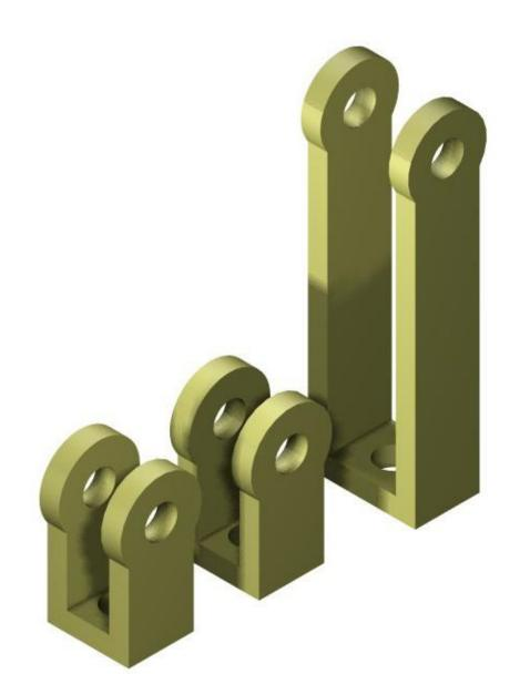
The completed clevises can be re-enforced by placing a small fillet of solder into the folded joints. Use solder sparingly and try not to fill the hole with solder. If you do fill the hole, just clean it out with a 0.5mm drill, as a wire needs to be located and soldered into the hole, in the next few steps. The main actuating rod from the base is 0.6mm, so drill a hole this size to accept the rod, in one of the small clevis's
