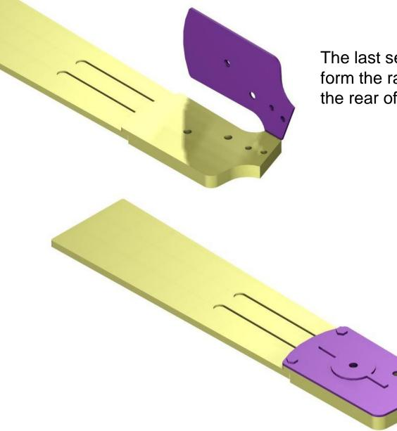
The last section should form the raised boss on the rear of the signal arm.
