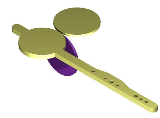
The discs are located top and bottom, to thicken up the weights of the arms. Solder the arms together once all is aligned.
