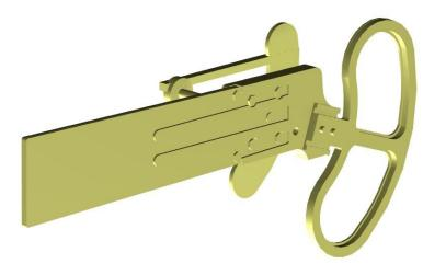
Locate and fix a length of 0.6mm wire through the hole in the signal arm ( the bearing plate may need to be drilled out to accommodate the wire.
