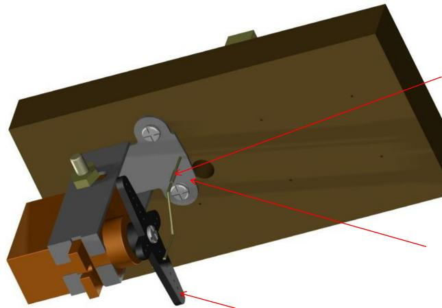
Make a coupler out of 1mm tube to join and adjust the brass wire rod. You can then glue or solder them in place
